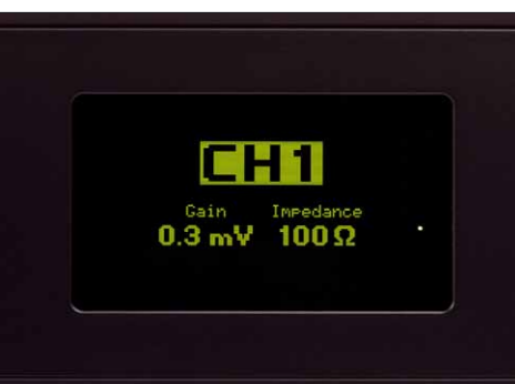
The „normal view“ of the display. It shows the selected input, the gain, and the input impedance
