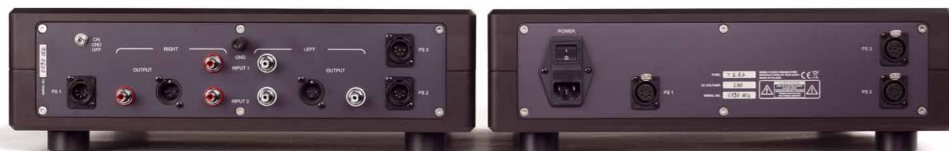
The Big Phono has two unbalanced pickup inputs
