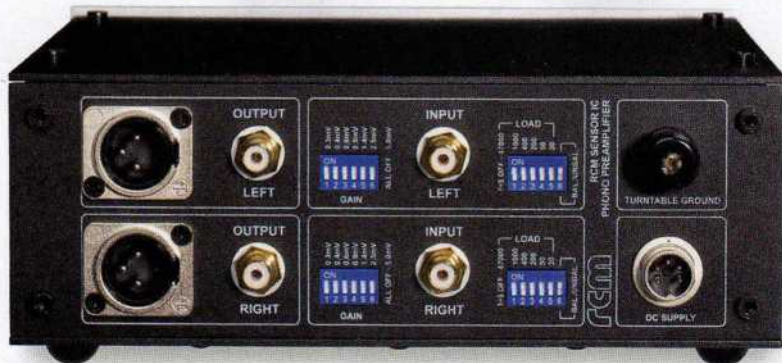
ABOVE: RCM offers a choice of seven input sensitivities from 5mV (MM) to 0.3mV (low output MC) plus a choice of six input loads from 47kohm down to 20ohm
